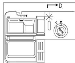
If the warning LED does not light up, you can estimate the amount of remaining rinse aid to the optical level indicator (D) next to the dispenser.
