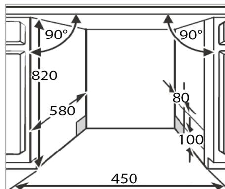
If the appliance is mounted in the corner of the cabinet base, sufficient space must be left to open the appliance door.
