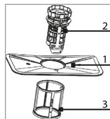
The three-part filter system prevents large quantities of food residues or foreign bodies from entering the rinsing system.
